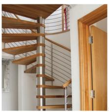
The Model 71 Spiral Staircase is a bespoke spiral stair, constructed with a steel centre column and timber treads. It is available in diameters from 1000-2400mm and can span multi levels if required. For strength, the timber treads are always hardwood, with beech, oak, maple, ash and walnut the most popular choices. It is a domestic spiral stair suitable for use as a primary or secondary staircase. Its modern, light and open appearance makes the Model 71 Spiral a real feature within a dwelling.
